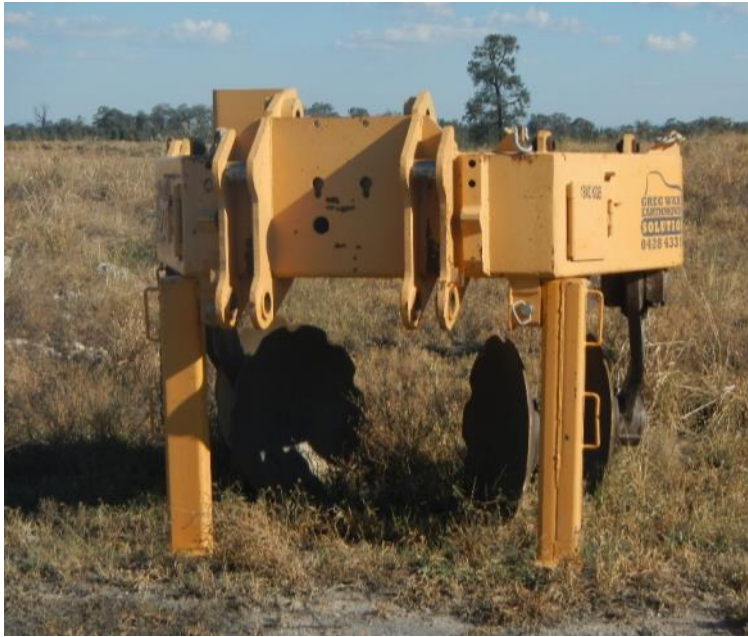
Figure 2. Mounding plough may also be used to create furrows and mounds
